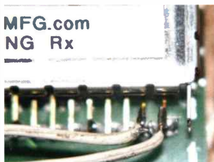
SCL and SDA lines soldered to the r.f. module.
