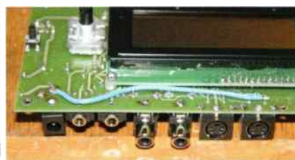
SCL and SDA lines soldered to the r.f. module.
