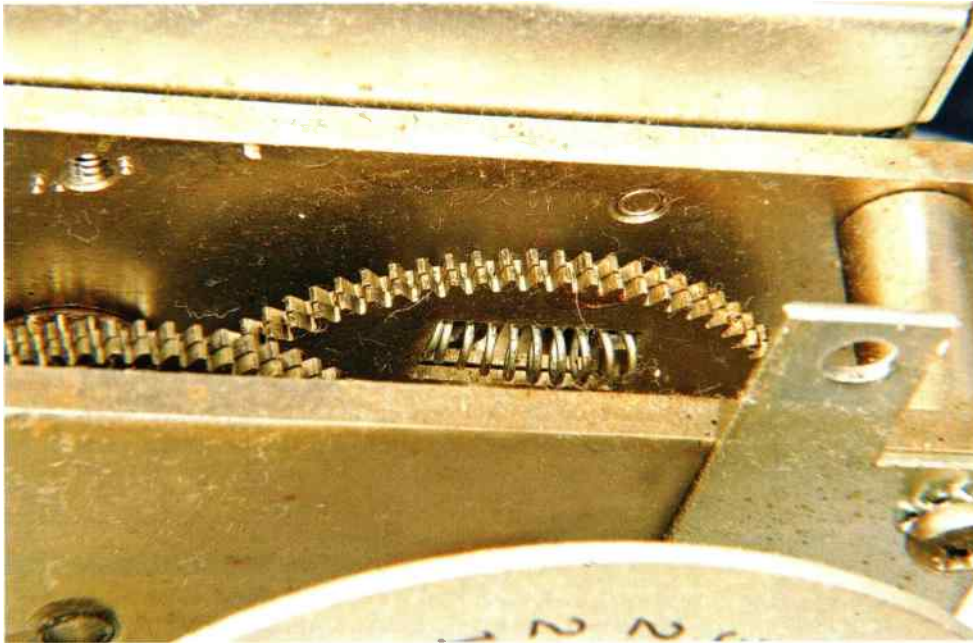
Fig. 7.4: Anti-backlash gearwheels have two half-width sets of gears held with a strong spring to counteract gear tooth wear.
