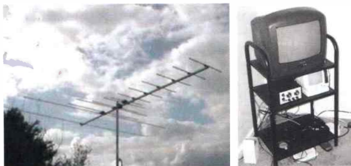
Fig. 11 (far right): Kevin Hughes' set-up with a D-100 converter feeding a Roadstar 10in portable. Indoor amplifiers from Antiference and Fringe Electronics are at the ready to connect when strong local broadcasts from the nearby Sutton Coldfield and Lichfield transmitters allow!
