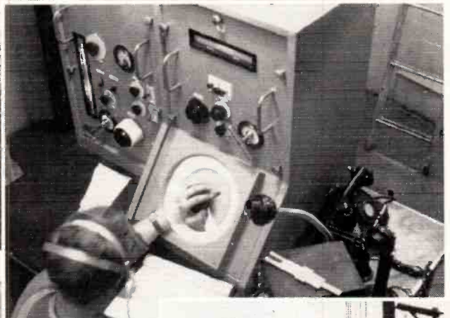
Fig. 4: Gerry Openshaw G2BTO, operating the d.f. station goniometer in 1943 showing the Marconi equipment. Three similar underground stations were at Wymondham in Norfolk, St. Erth in Cornwall and Thurso, Scotland.
