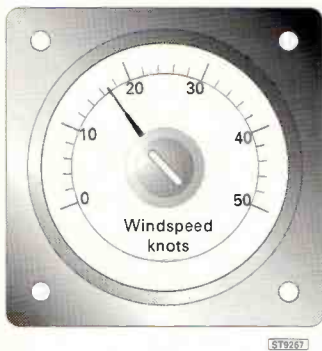
Fig. 5: The meter scale should be calibrated to about 60 knots.
