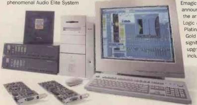
The new ProToolsi24 MIX (in foreground) combines I/O and DSP on a card
