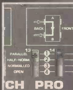
Detailed view of a section. With the switch you choose the operating mode:
