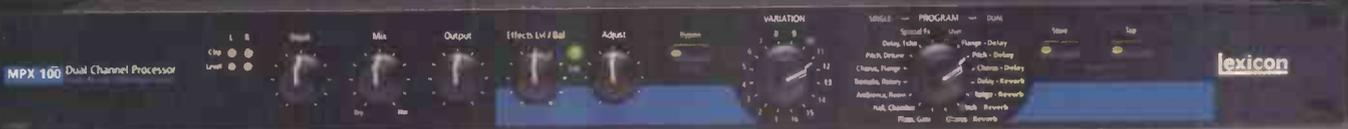
The MPX 100 is a true stereo dual-channel processor with 24-bit internal processing, 20-bit A/D-D/A and S/PDIF digital output for a very affordable price. Powered by a new version of Lexicon's proprietary *Lexichip*™ the MPX 100 has 240 presets with classic, true stereo reverb programs such as *Ambience*, *Plate*, *Chamber* and *Inverse* as well as *Tremolo*, *Rotary*, *Chorus*, *Flange*, *Pitch*, *Detune*, 5.7 second *Delay* and *Echo*. Dual-channel processing gives you completely independent
