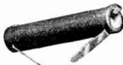
Three type 36EH60 rectifiers, each only 3½" long X ¼" dia, will, from a peak pulse input of approx. 4,500V obtained from the standard line scanning output transformer, give an output of about 10kV at 100µA, used in the tripler circuit shown on the left.
