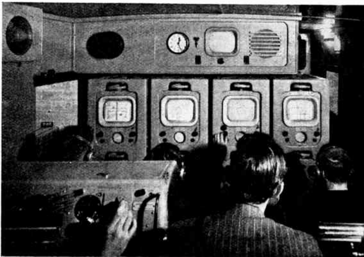
O.B. TELEVISION. —Interior of the O.B. van equipped by Pye to B.B.C. specification. Three of the four rack-mounted tubes monitor the three Photicon cameras and the fourth the picture transmitted from the van. The image received from A.P. is shown on the upper tube.
