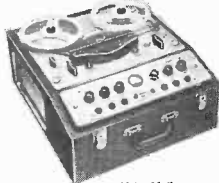
MARK 5 TYPE M SERIES 3 MONO—HALF TRACK—THREE HEADS— RECORDING LEVEL METER Separate record and playback heads—separate record and playback amplifiers—amplifier frequency response 25–28,000 c/s ±3dB—power output 2 watts r.m.s.—separate bass and treble controls—mixing of input signals—speaker monitoring whilst recording.
