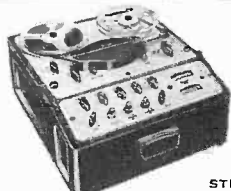
STB2 MONO/STEREO—HALF TRACK (Record/ playback)—QUARTER TRACK (playback) FOUR HEADS—TWO EDGEWISE METERS Designed for use with high fidelity stereo installations—adjustable attenuators on all input channels to ensure perfect matching with all auxiliary equipment—dual concentric recording level and playback level controls—cathodic follower output—four channel mixing on mono programme sources—twin recording and twin playback pre-amplifiers—comparison of original and recorded signal—adjustable bias level—recording facilities for 1/2 and 2/2 track—playback facilities for 1/2, 2/2, 1/4 and 2/4 tracks—sound-on-sound facilities—two edgewise meters for recording level, tape output level and bias level. Optional extra: stereo power amplifiers and monitoring speakers.
