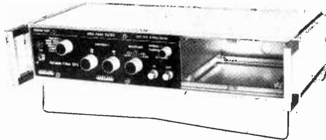
EF3-05 High Pass Cut-off frequency variable from 1Hz to 1MHz
