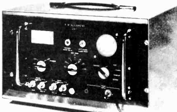
The F.M. Alignment Unit Type FMU/1 illustrated was designed at the Royal Radar Establishment, Malvern, to suit Amplex Recorders working on the IRIG intermediate band specification (using ES 100 Electronics) e.g. Model Numbers FR 1200, FR 1260, FR 1300, FR 1800L, FB 400, PR 500
