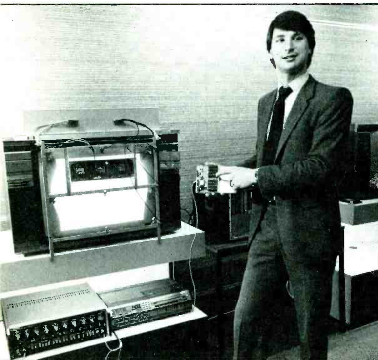
This automatic alignment system cuts out costly factory adjustments. A grid of light sensors over the screen responds to a sequence of test waveforms generated by a microcomputer system. The equipment handles picture-geometry and white-point adjustments and it programmes the appropriate control settings into the tv set's internal microcomputer.
