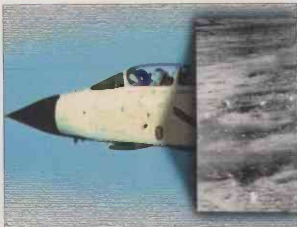
Fig. 1. Mechanically-scanned television is in use today by the military. In airborne reconnaissance, the high-resolution television cameras on RAF Tornado GR1A aircraft use mirror-drum scanning. Coincidentally the aspect ratio is similar to that of Baird's 30-line standard. (from Crown Copyright original)
