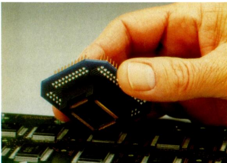
ITT test clips ease in-situ testing of PQFP surface mount devices.
