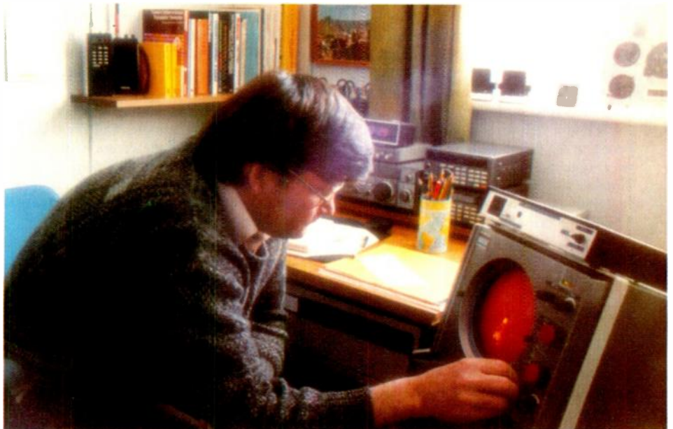
Mk III display system: Decca 101 display and, on top, the digital display drive generator
