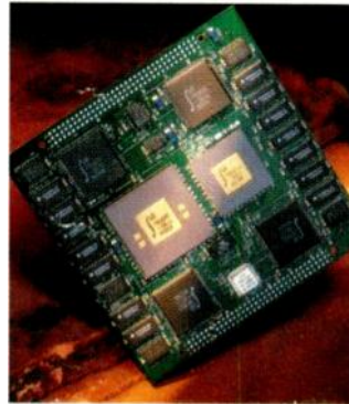
Risc subsystem module from IDT implements R3000 architecture.
