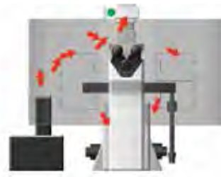
Fig. 1–Single air input and no venting causes random air flow in a traditional incubator.
