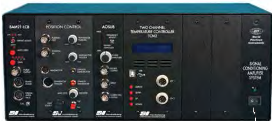
SI-BAM21-LCB Optical Transducer Amplifier SI-CISB Position Control Module SI-AOSUB Anti Oscillation Unit SI-TCM2B Temperature Control Module Expansion Slots Power Switch
