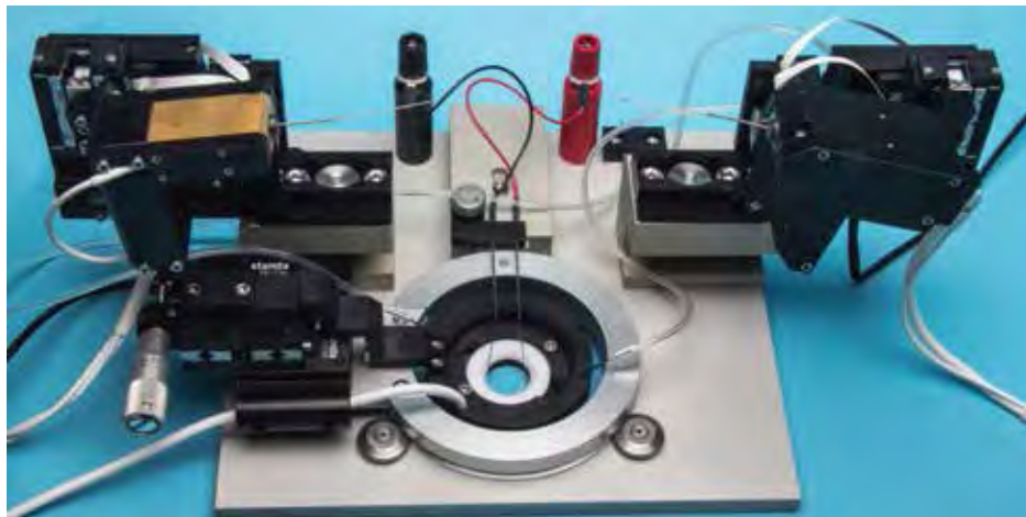
The manipulators tilt up and fold back to facilitate system setup. There are two programmable memory positions (home and target) for easy exchange of the 35mm dishes, providing access to the bath so you can add the live cells. The combination of these features enables high experimental throughput.
