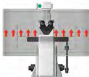
Fig. 3–A diffusion grid with air input and exhaust vents yields consistent air flow.
