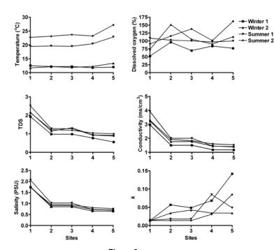
**Figure 2** Temperature (°C), dissolved oxygen (%), total dissolved solids (TDS), conductivity (ms/cm<sup>3</sup>), salinity (PSU) and water transparency (k) at each site within the Sundays River
