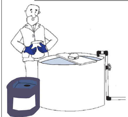
✓ The operator sometimes has to mix the flocculant in a beaker first
