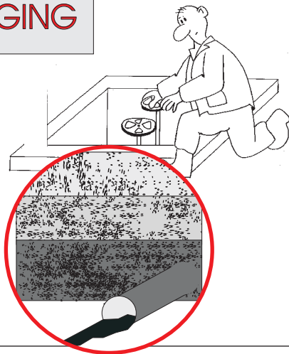
The operator removes the sludge from the sedimentation tank with the desludge valve. This should be done at least once every shift
