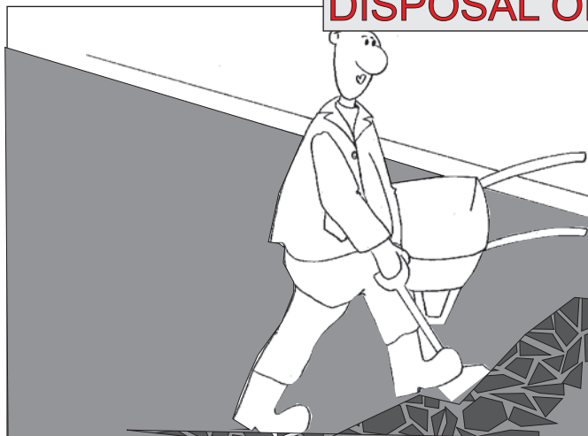
The operator removes the dried sludge
