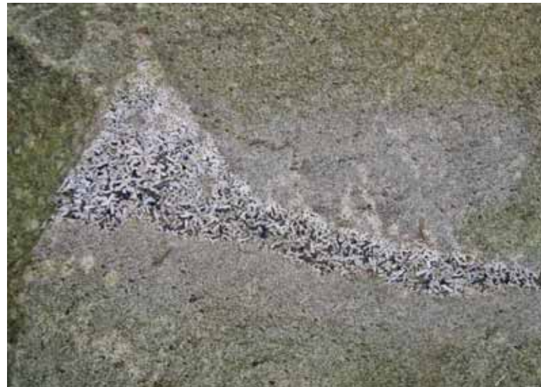
Pegmatite vein in a microsyenite spall (actual size 300mm x 387mm)
