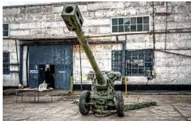
Metinvest workers replicate bulky machinery from lightweight materials. Above, a full-size mock-up of the D-20 gun-howitzer.
