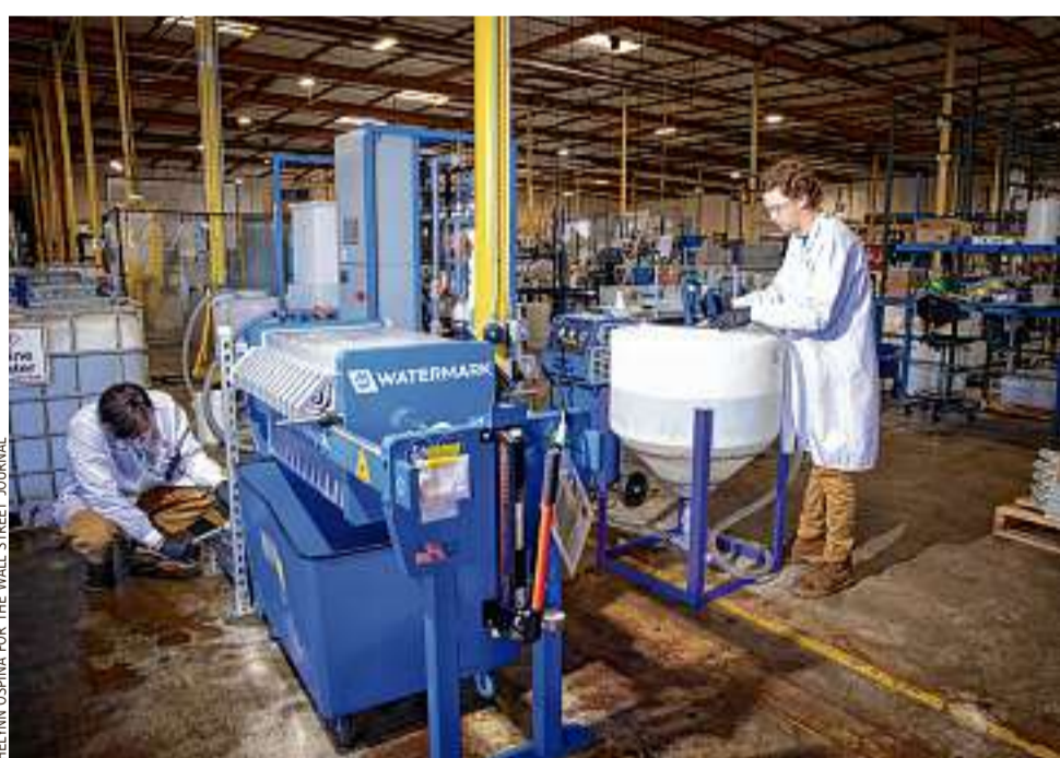
Lilac uses reusable ceramic 'beads' that attach to lithium atoms to free them from the brine.
