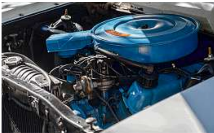
The 302-cubic-inch V-8 engine puts out 210 horsepower, the car's original brochure says.
