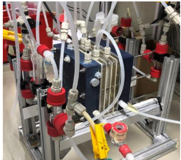
Figure 2: Microbial electrolysis cell removing ammonium from wastewater.
