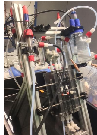
Fig 2. Laboratory setup of a bioelectrochemical chain elongation system.
