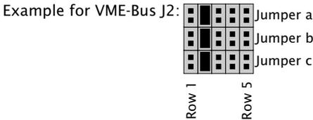
Use the following table to determine how jumpers a-c in the corresponding row depending on which bus system is used.
