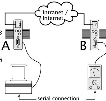
**Example 3:** A control program polls multiple measuring devices; the measuring devices can (e.g. in case of error) independently send data to the control program.
