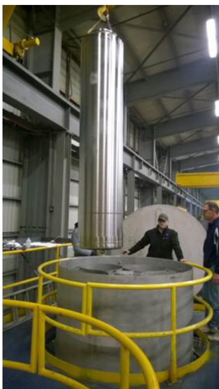
Loading Test Canister into an Overpack
