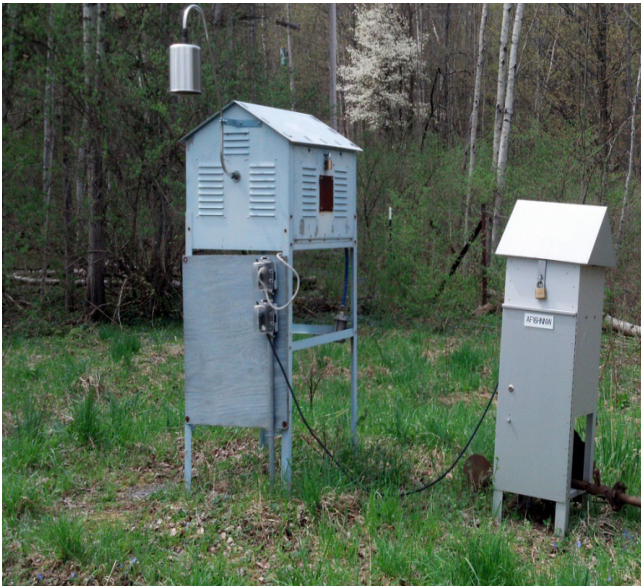
Low-Volume and High-Volume Samplers Located in the Historical Predominant Downwind Direction from the Site
