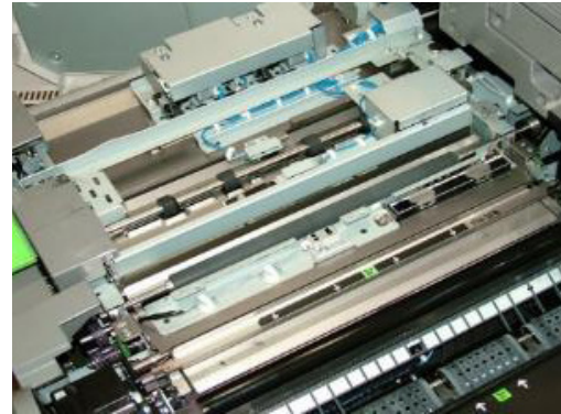
The Aligner Transport helps register the paper to +/- 0.5 mm.
