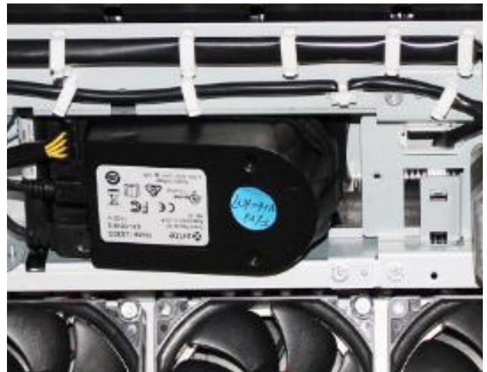
The X-Rite® Inline Spectrophotometer automates the collection of XRGB data for calibration and profiling.
