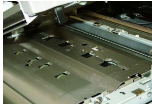
A Registration Gate de-skews the paper and then drops as the sheet advances to the Contact Image Sensor for additional adjustment.
