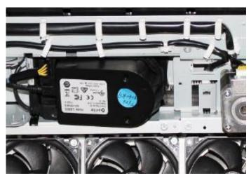
The X-Rite  $^{\otimes}$  Inline Spectrophotometer automates the collection of XRGA data for calibration and profiling.
