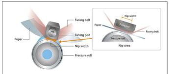
Fuser Belt Pressure and Heat Control
