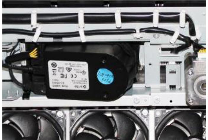
The X-Rite® Inline Spectrophotometer automates the collection of XRGB data for calibration and profiling.
