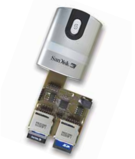
Figure 7 – Xilinx demo board plugged into a USB SD card reader
