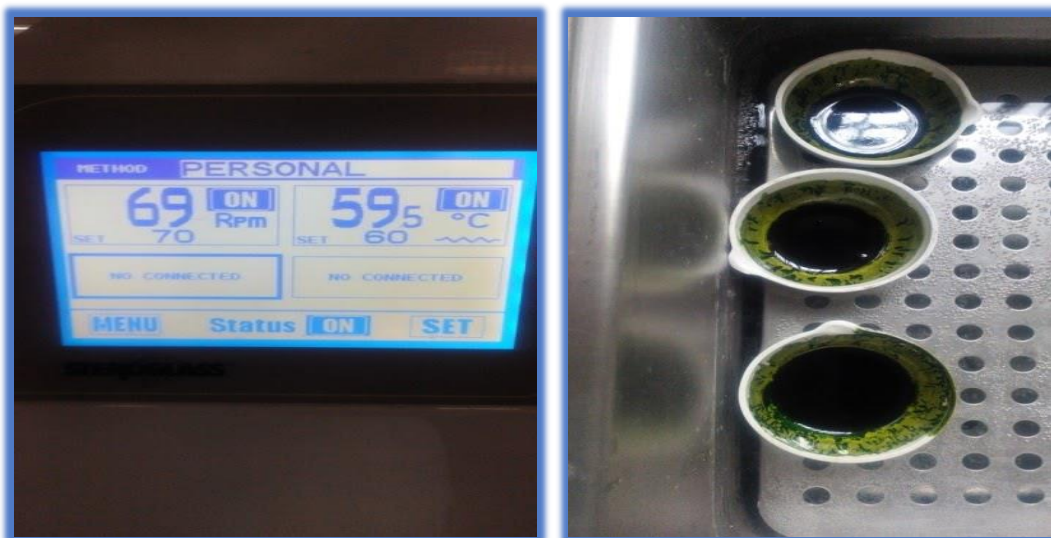
Figure 4: Shows extract passing through rotary vacuum evaporator for the separation of solvents extract in water bath for complete evaporation of solvents.
