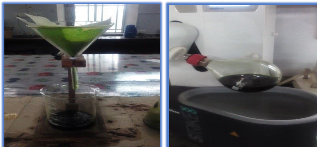
Figure 3: Shows filtration of the extract separation (Rotary vacuum evaporator) of solvent from crude extract.
