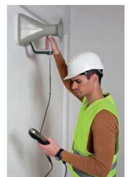
Aerolics performance measurement with a balometer
