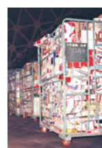
14—Roll box pallets (or roll containers) with caster wheels used for department store deliveries
