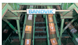
12—Automated parcel sorting machine manufactured by Sandvik (circa 1990)
