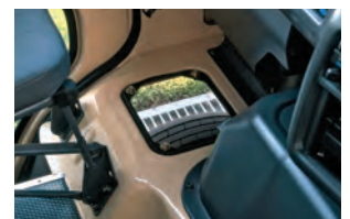
6—"Cat Window" installed below the driver's seat
