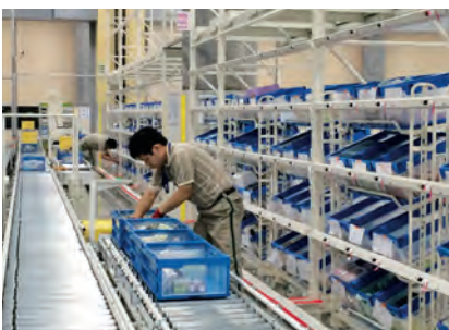
14—Free Rack Auto Pick System (FRAPS) in use at Atsugi Gateway
