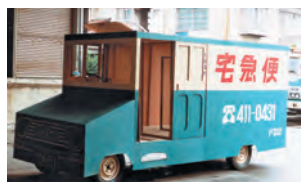
3—Prototype TA-Q-BIN pickup and delivery vehicle made from plywood (March 1980)
