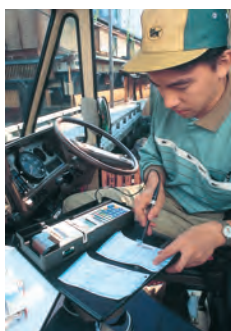
11—3rd Generation NEKO System with pen scanner attached to portable POS (PP) terminal enabled more accurate entry of information at the customer's front door (1990s)
