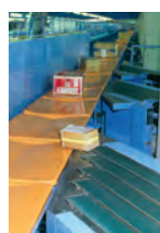
13—Tray-based automated parcel sorting machine (Osaka Regional Branch, 1985)
