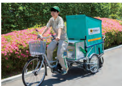
18—Electric bicycle with trailer used for parcel pickup and delivery (2015)
