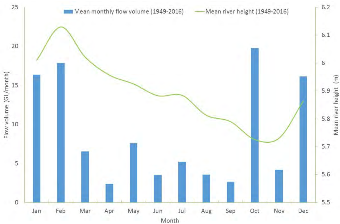
Figure 4 Flow volume and river height for Dogwood Creek at Gilweir (DNRM station 422202B, located approximately 5 km south of Miles)
