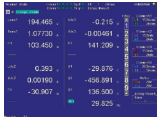
Example of DC voltage, current, and power at three points and conversion efficiency measurement.
