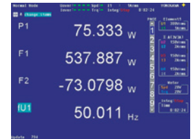
Example of power (P1) and instantaneous peak power on the plus (F1) and minus (F2) sides
