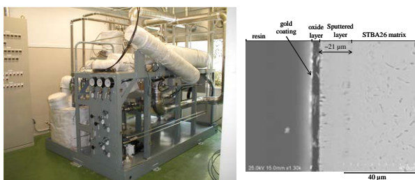
Fig. 7 Corrosion test loop and Al-Fe alloy-coated steel
