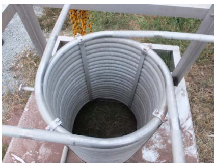
Fig. 1 Heat absorber tubes used at the test site
