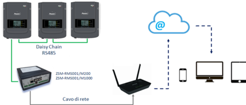
Figure 94 – Diagram showing the operation of the ZSM-RMS001/M200 / ZSM-RMS001/M1000 datalogger
