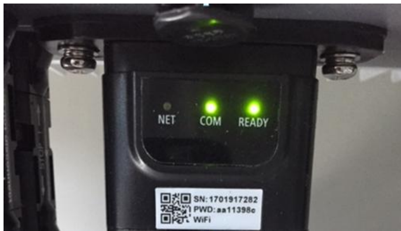
Figure 83 - Initial status of LEDs
