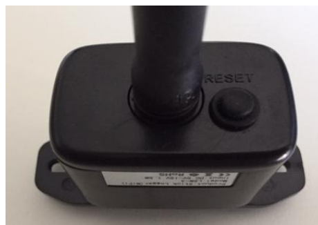
Figure 73 – Reset button on the Wi-Fi adapter
