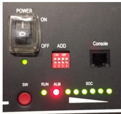
Figure 50 - Battery status after setting the POWER switch to ON and pressing the SW button
