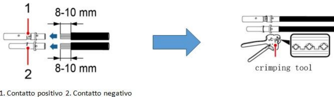
Figure 41 – Preparing the positive and negative photovoltaic cables
