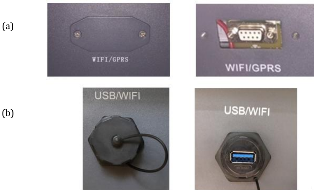
Figure 54 - Port for external Wi-Fi adapter
