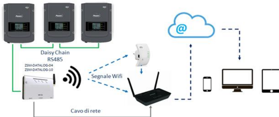
Figure 93 - Diagram for connecting the ZSM-DATALOG-04 / ZSM-DATALOG-10 datalogger
