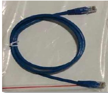
Figure 37 – Communication cable between AZZURRO 5000 batteries
