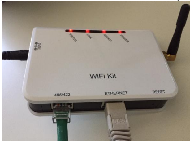
Figure 101 - Ethernet cable connected to the datalogger
