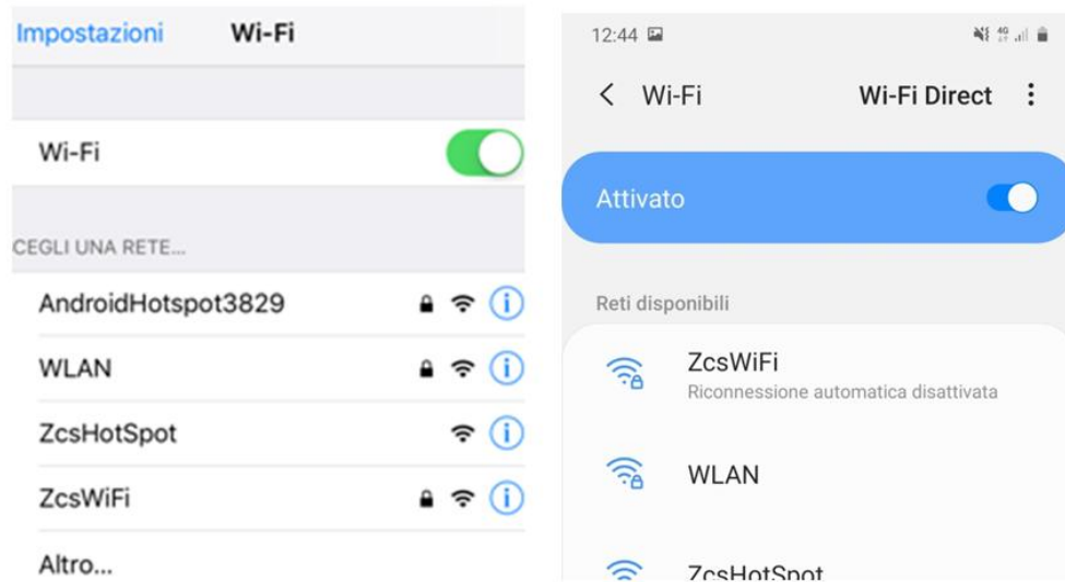
Figure 69 – Wi-Fi network search on Smartphone (iOS and Android); Access point of the Wi-Fi adapter is no longer visible
