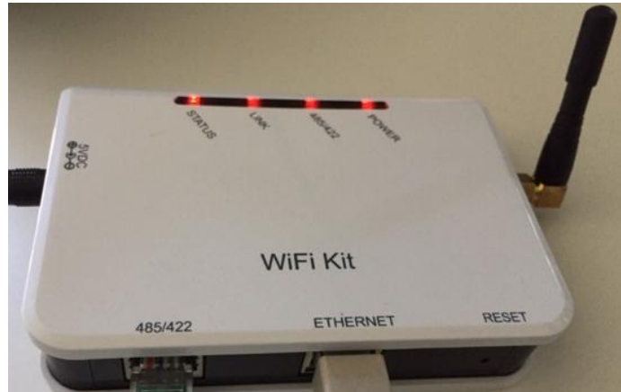
Figure 114 – LED indicating the correct configuration of the datalogger
