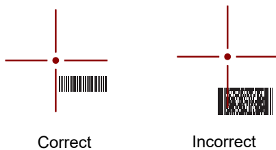
Figure 3-5 Imager Aiming Pattern: Bar Code Not Centered
