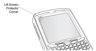
Figure 6-1 Removing the Screen Protector
