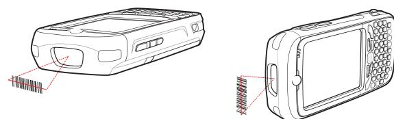
Figure 3-1 Linear Scanning
