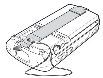
Figure 1-11 Handstrap Clip Removal
