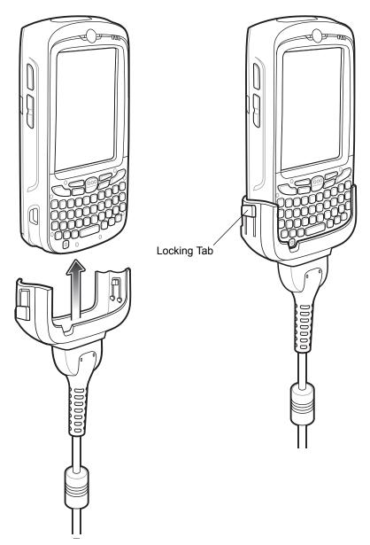
Figure 5-11 Cable Cup Locking Tabs
