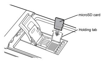
Figure 1-4 Insert microSD Card in Holder
