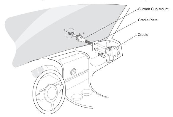
Figure 5-13 Windshield Installation
