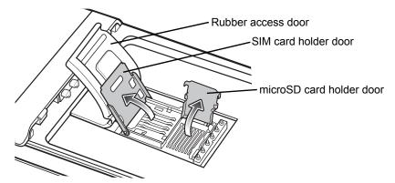
Figure 1-3 Lift SIM Slot Holder Door
