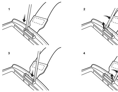
Figure 1-12 Handstrap and Pin Removal
