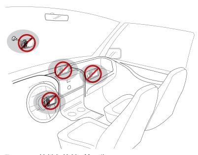
Figure 5-12 Vehicle Holder Mounting
