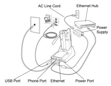
Figure 5-3 Connection Setup
