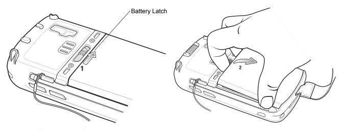
Figure 1-8 Removing the Battery
