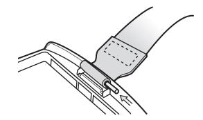
Figure 1-14 Feed Handstrap into Handstrap Slot
