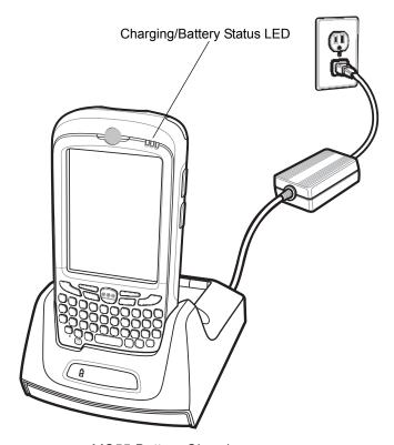
Figure 5-1 MC55 Battery Charging
