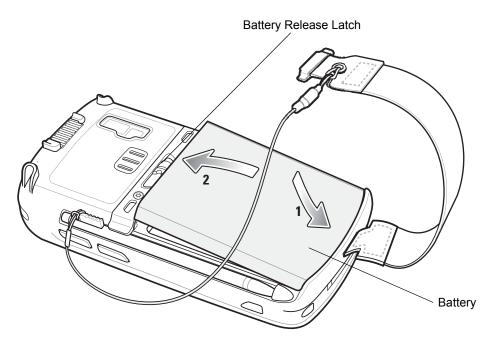
Figure 1-7 Inserting the Battery
