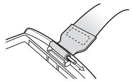
Figure 1-13 Pin Removal
