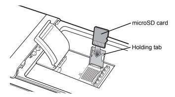
Figure 1-6 Insert microSD Card in Holder
