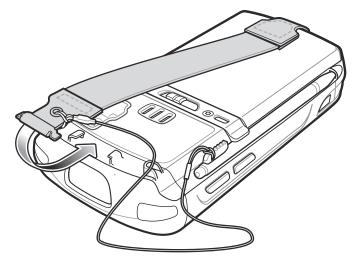
Figure 1-16 Slide Handstrap and Tether Over Handstrap Mount
