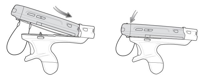
Figure 5-18 Installing the MC55
