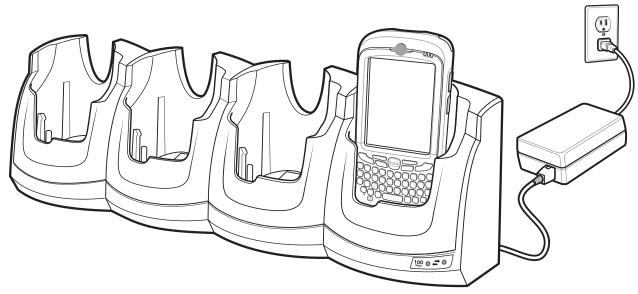
Figure 5-7 MC55 Battery Charging
