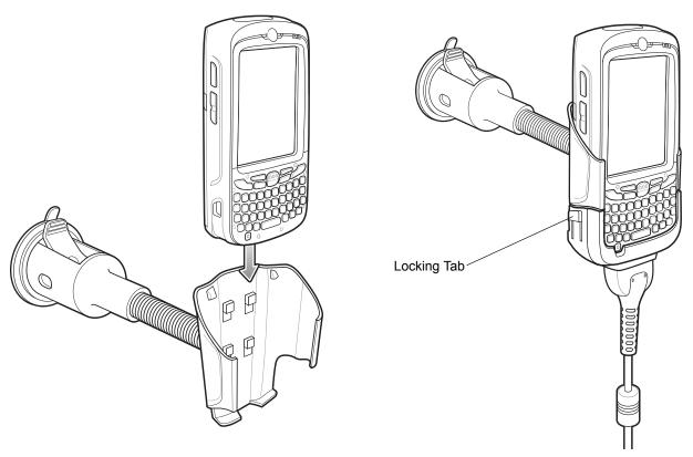
Figure 5-14 Insert MC55 into Vehicle Holder
