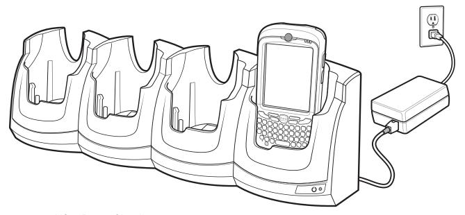
Figure 5-6 MC55 Battery Charging
