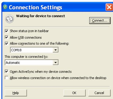
Figure 4-10 ActiveSync Connection Settings
