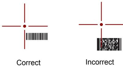
**Figure 3-5** Imer Aiming Pattern: Bar Code Not Centered
