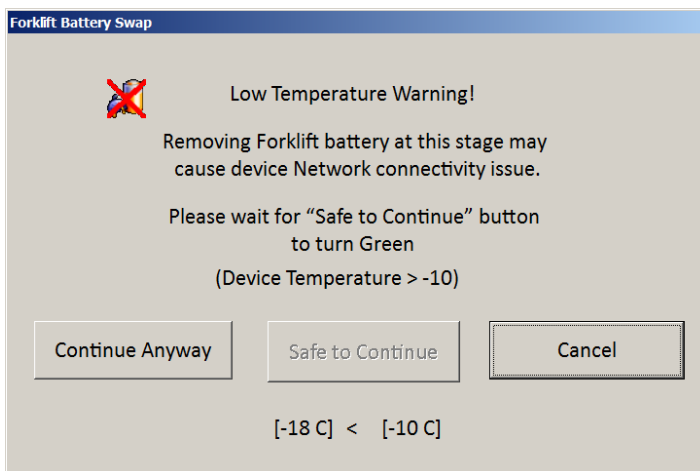
Figure 2-2 Forklift Battery Swap - Low Temperature Warning
