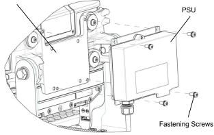
**NOTE** You need to also use an extender cable PN 25-159549-01 to connect the PSU to the vehicle computer.
