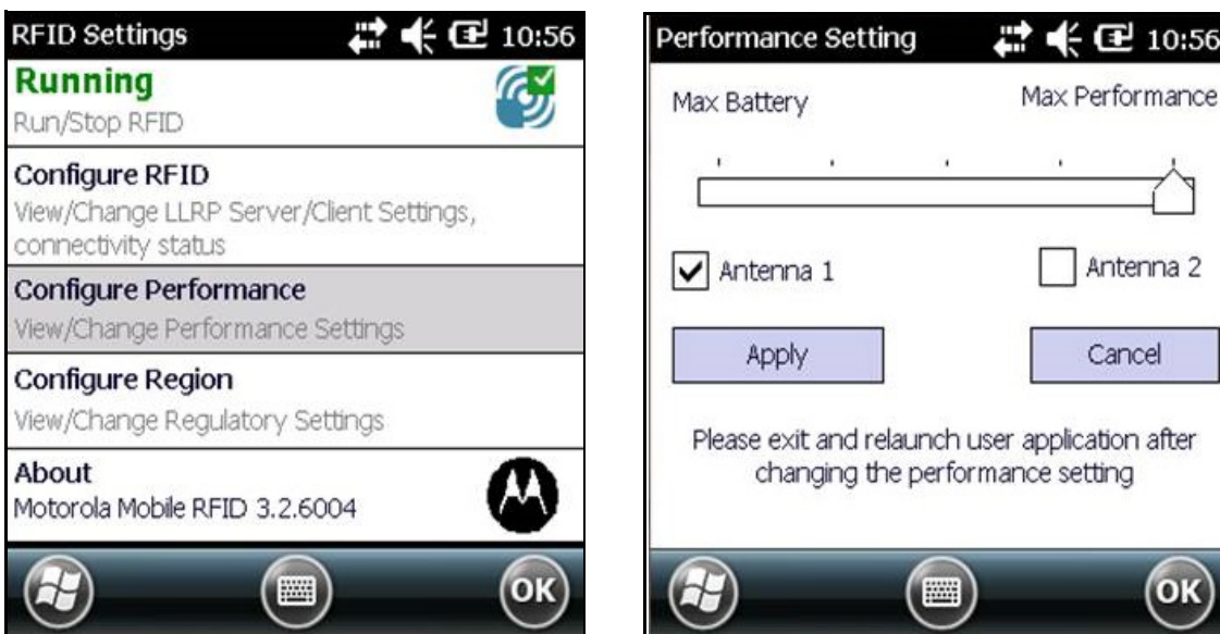
Figure 3-13 Battery Performance Configuration
