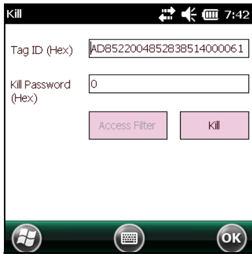
Figure 4-19 Kill Access Operation Window
