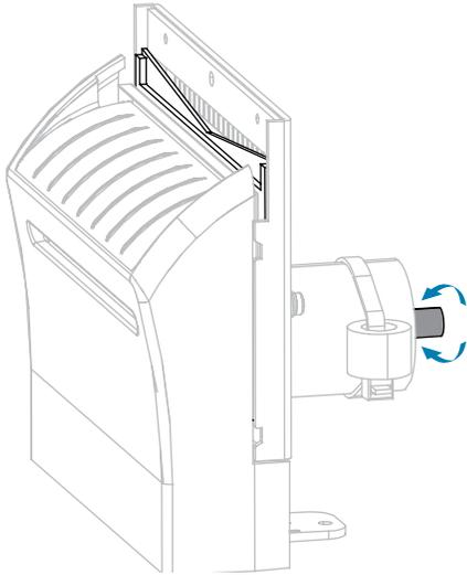
7. Using the swab from the Preventive Maintenance Kit (part number 47362), wipe along the upper cutting surface (1) and the cutter blade (2). In place of the Preventive Maintenance Kit, you may use a clean swab dipped in 90% isopropyl alcohol. Allow the solvent to evaporate.
