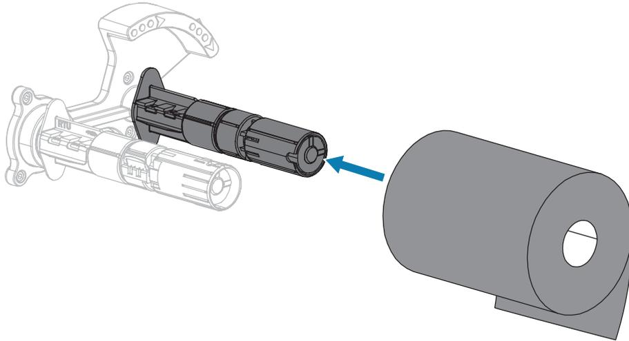
4. Your printer shipped with an empty ribbon core on the ribbon take-up spindle. If this core is no longer there, place an empty ribbon core on the ribbon take-up spindle. Push the core back as far as it will go.
