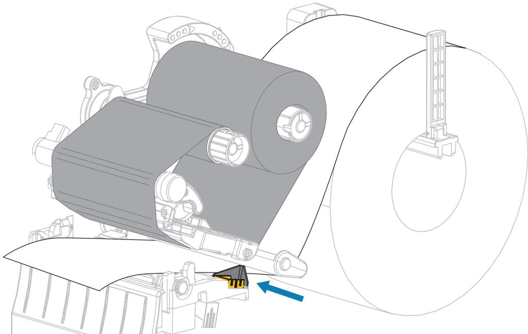
2. Rotate the printhead-open lever downward until it locks the printhead in place.
