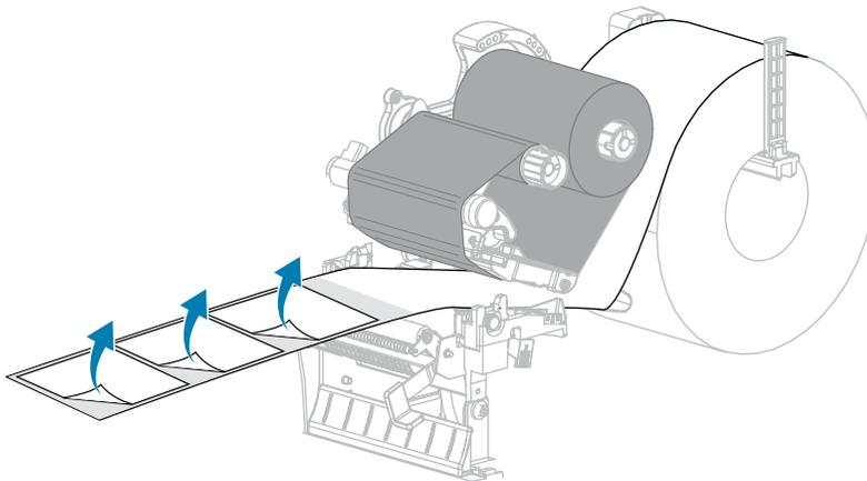
5. Pull the media into the printer so that only the backing is between the media sensors.
