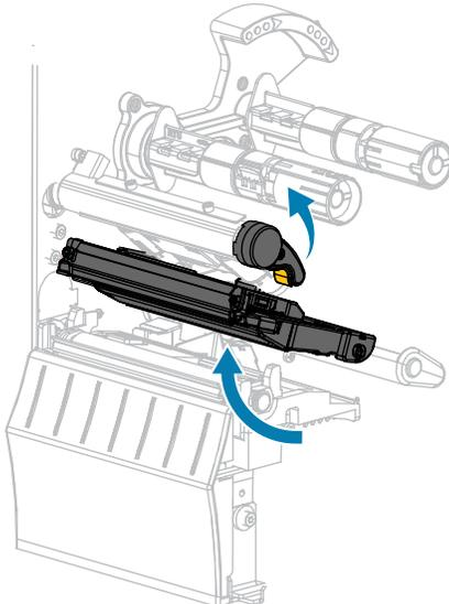
3. Place the roll of ribbon on the ribbon supply spindle with the loose end of the ribbon unrolling as shown. Push the roll back as far as it will go.
