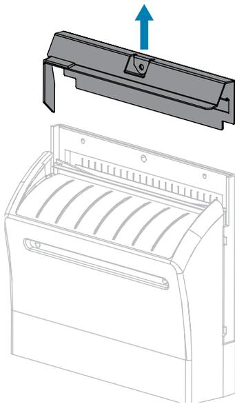
6. If necessary, rotate the cutter motor thumbscrew to fully expose the V-shaped cutter blade.
