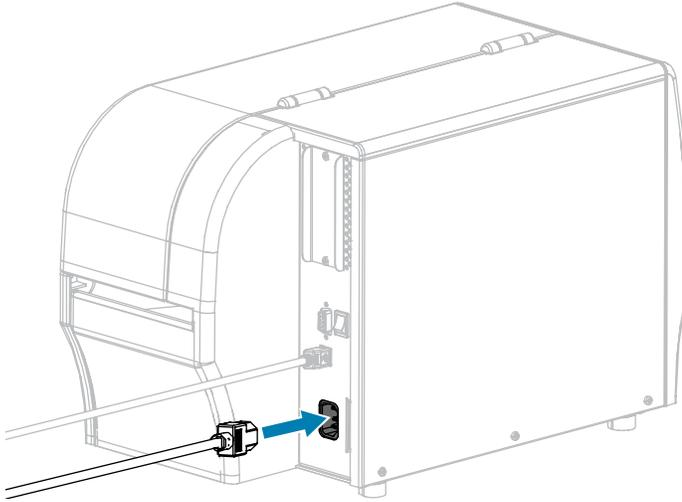
4. Plug the A/C power cord into an appropriate power outlet.
