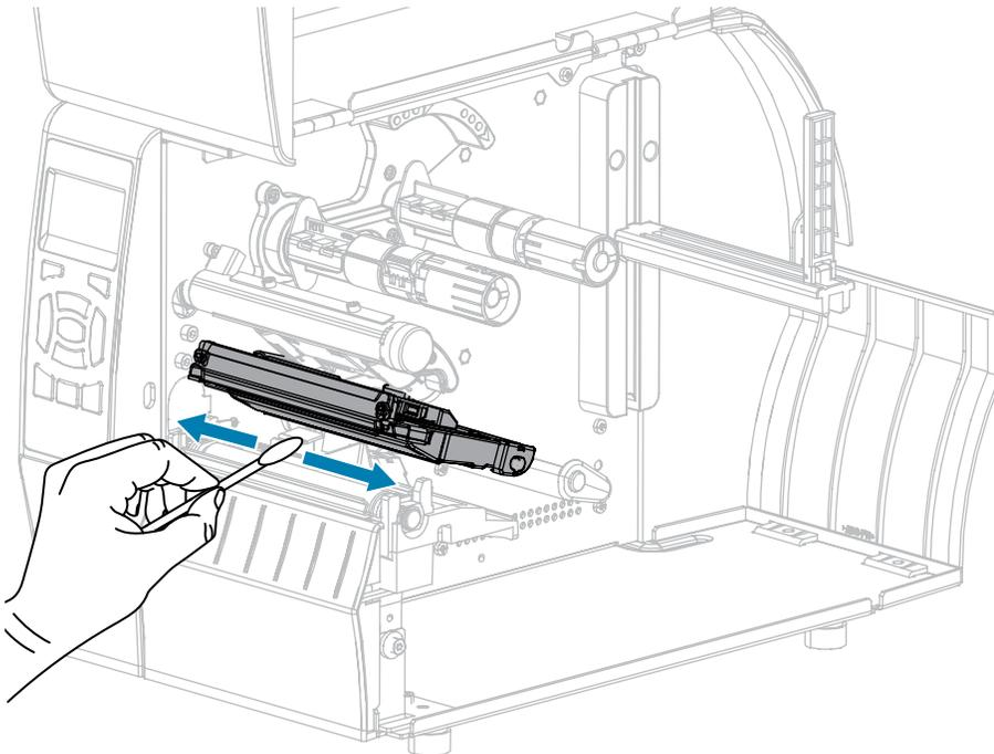
5. While manually rotating the platen roller, clean it thoroughly with the swab. Allow the solvent to evaporate.
