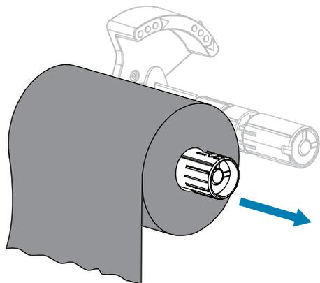
3. Discard the used ribbon. You may reuse the empty core from the ribbon supply spindle by moving it to the ribbon take-up spindle.
