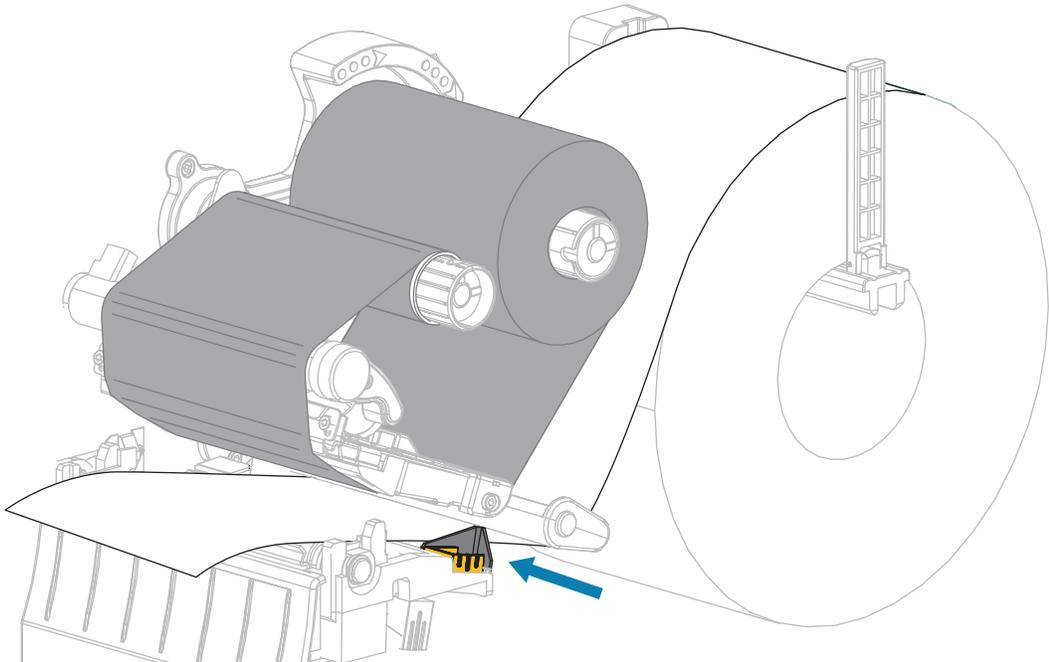
8. Rotate the printhead-open lever downward until it locks the printhead in place.
