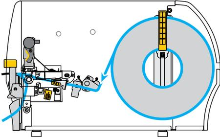
1. Push down the peel-off mechanism release lever to open the peel assembly.
