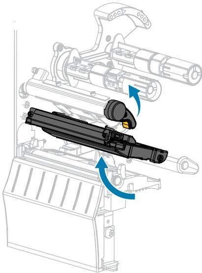
3. Insert media into the printer. Follow the instructions for roll or fanfold media, as appropriate.
