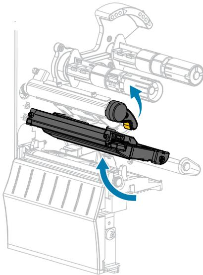
3. Push down the peel-off mechanism release lever to open the peel assembly.
