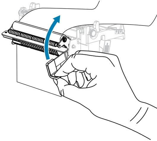
9. Rotate the printhead-open lever downward until it locks the printhead in place.
