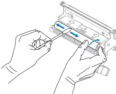
6. Use the swab to remove excess adhesive from the tear-off/peel-off bar. Allow the solvent to evaporate.
