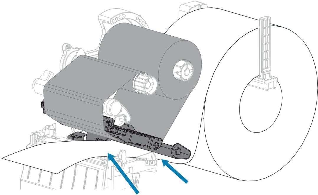
6. Make sure that the media passes through the slot in the transmissive media sensor (1) and under the inner media guide (2).
