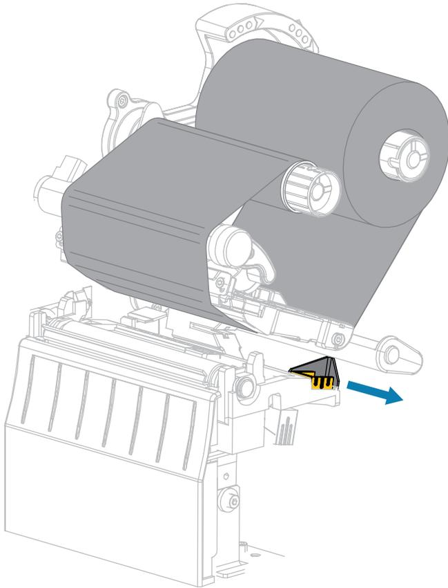
5. Slide the media under the media dancer assembly and the printhead assembly. Allow the end of the media to extend out of the front of the printer.
