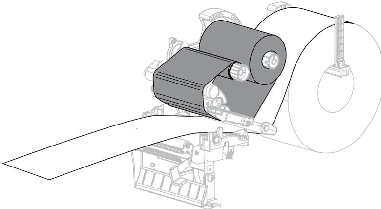
4. Remove the exposed labels so that only the liner remains.
