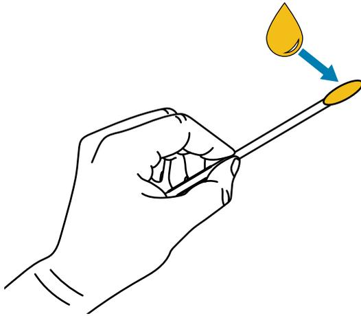
9. Apply an even layer along all exposed surfaces of both cutter blades. Remove any excess oil so that none of it comes in contact with the printhead or platen roller.
