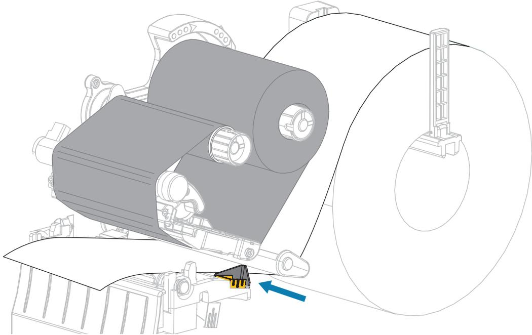
3. Rotate the printhead-open lever downward until it locks the printhead in place.
