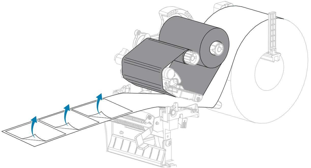
4. Feed the liner behind the peel assembly. Make sure that the end of the liner falls outside of the printer.
