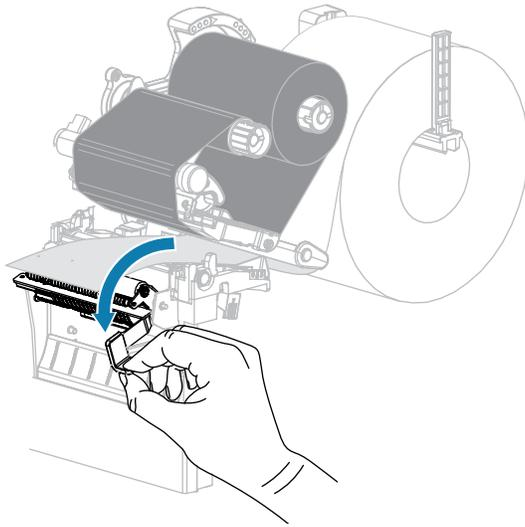
4. Remove any media liner to expose the pinch roller.
