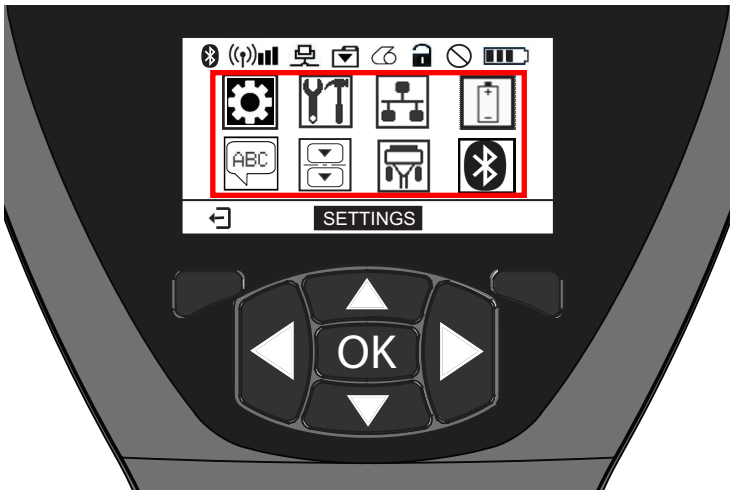
Figure 17: Home Display Screen (QLn420 and QLn Healthcare)
