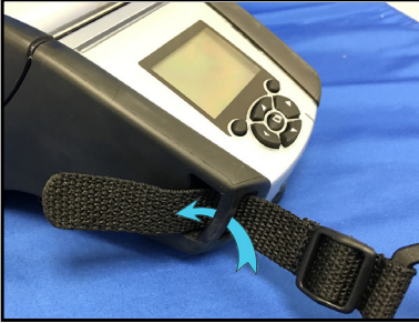
Figure 30: Using the Optional Shoulder Strap
