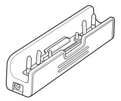
1. Align the pins in the Rugged Charge Connector with the slots in the ET5X.
