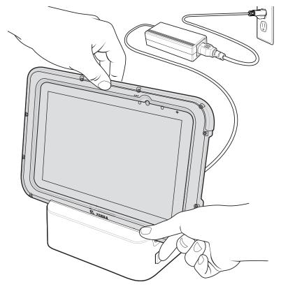
Figure 91 Remove ET5X from Rugged Communication and Charging Cradles
