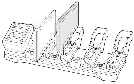
3. Place the ET5X down into the slot with display facing away from Battery Charger.
