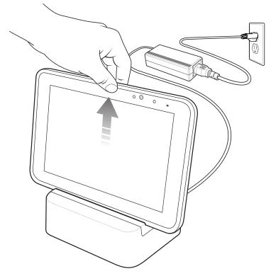
Charge batteries in ambient temperatures from 0°C to 40°C (32°F to 104°F) as reported by the battery. Charging is intelligently controlled by the charger. To accomplish this, for small periods of time, the charger alternately enables and disables battery charging to keep the battery at acceptable temperatures.
