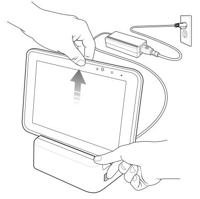
Figure 86 Remove ET5X from Communication and Charging Cradles
