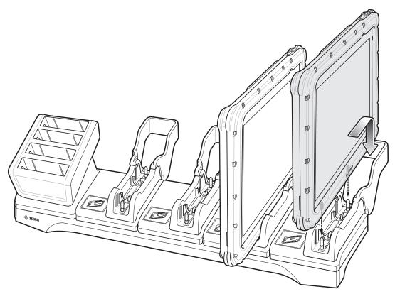
3. Place the ET5X down into the slot with display facing away from Battery Charger.
