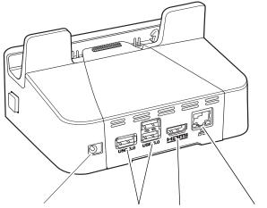
Power Input USB 3.0 Ports HDMI Port LAN (RJ45) Port
