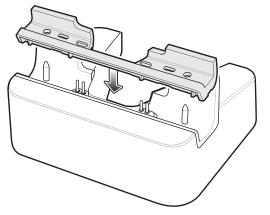
2. Press the insert down until it seats flush in the cradle.
