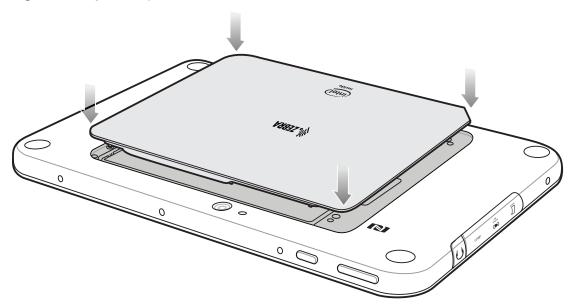
9. Carefully press down around the edge of the cover. Make sure that the cover is seated properly.
