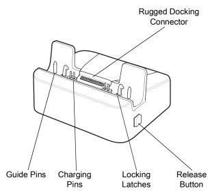
Figure 88 Rugged Communication and Charging Cradle - Rear View
