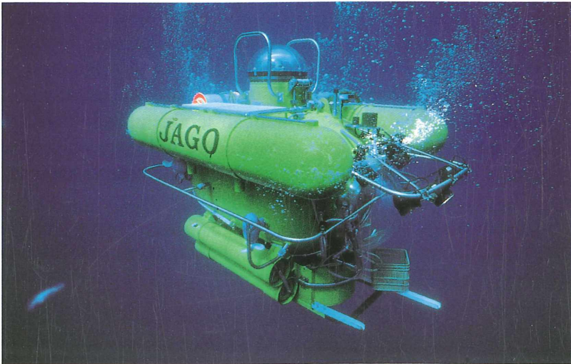
Fig. 1: Two-man-submersible "Jago" with depth capacity of 400 m. The weight of the craft is 3.3 tons.
