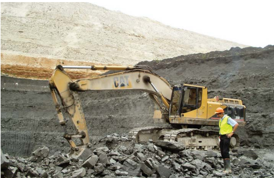
Left Chalk and Gault clay are blended to make cement at Ferriby in North Lincolnshire.
