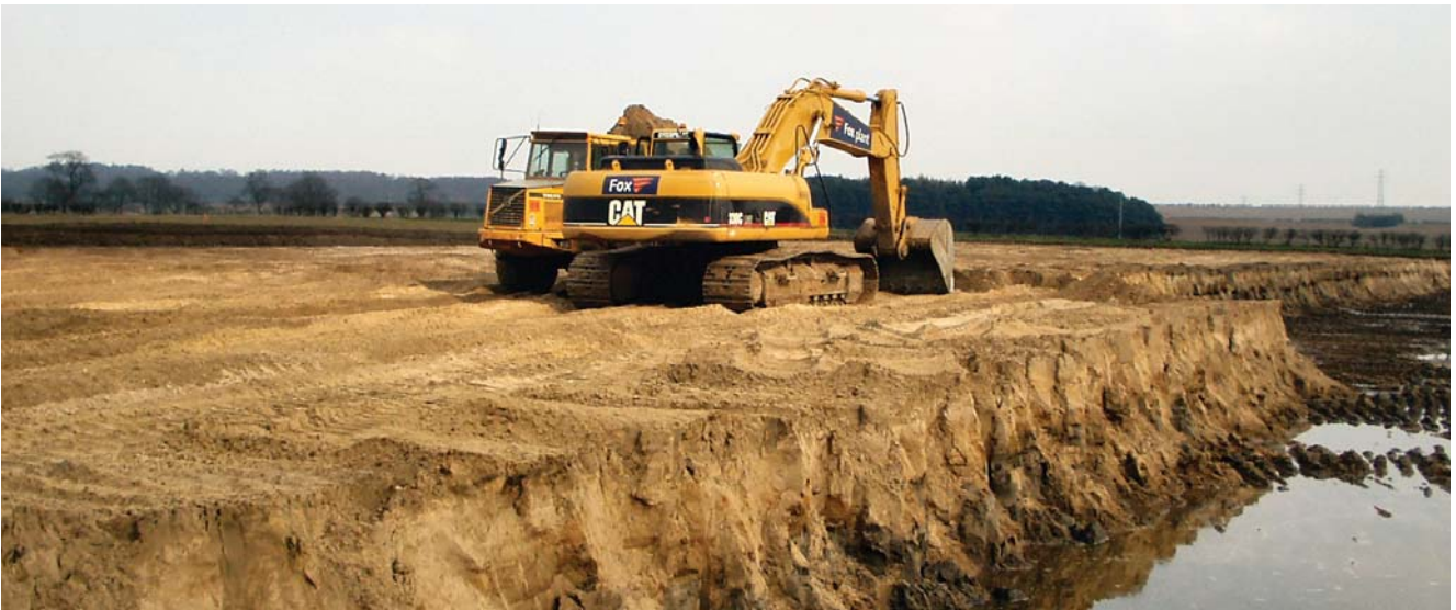
Above Thin, but extensive spreads of wind-blown silica sand are worked at Messingham in North Lincolnshire for use in a range of products including container glass.
