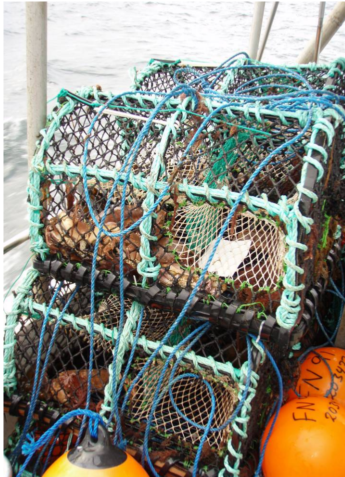
Figure 2.6. 'Scottish type' lobster/crab trap with dimensions 66 x 47 x 42 cm. Photo: Claus Stenberg.
