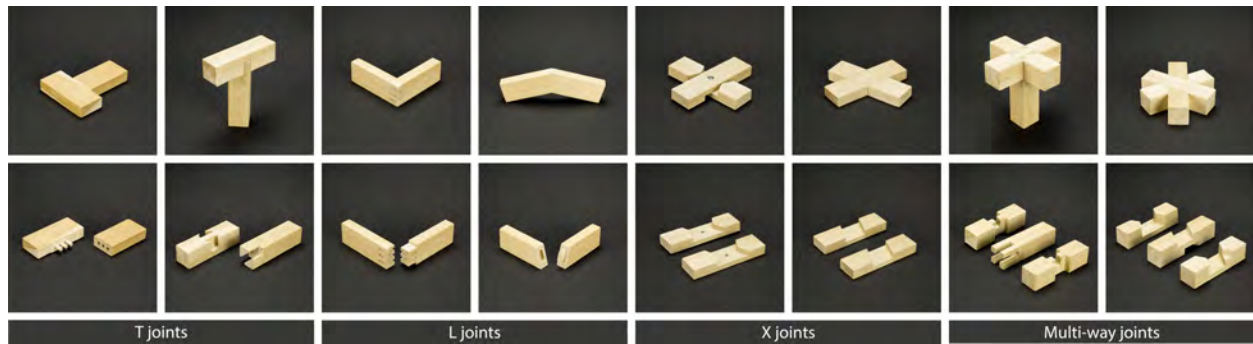
Figure 3.7: We categorize the joints our machine can create based on the orientation in which they come together. Top row shows assembled joints, bottom row shows disassembled joints. From left to right: dowel pin joint, framing joint, finger joint, angled mortise and tenon, pivoting lap joint, angled lap joint, three way interlocking tenon joint, and three way lapped joint. All example joints are created from poplar.
