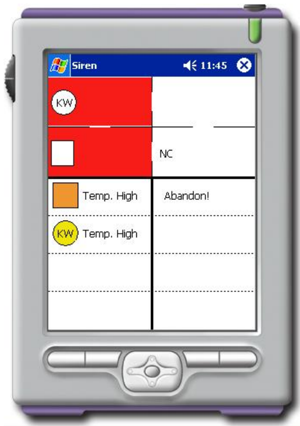
Figure 4. User Interface for Siren-based Context-aware Messaging Application. The upper part of the interface is a floor plan with four adjacent rooms. The lower left part contains user alerts generated by Siren, and the lower right part contains messages manually generated by fellow firefighters or incident commanders.
