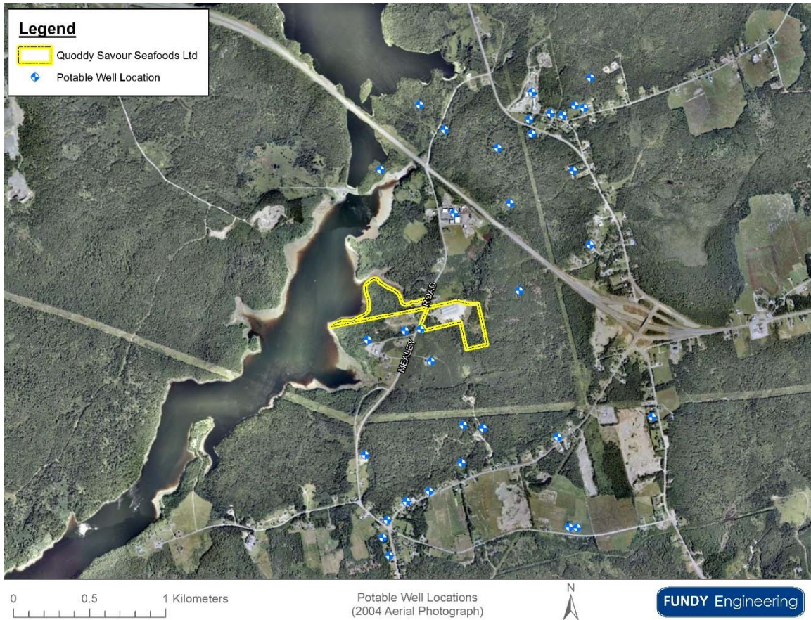
Figure 16. Aerial photograph showing groundwater wells on file with the NBDELG within a 1.5 km radius around PID 15160708 in Pennfield, New Brunswick. The well logs and water quality records were obtained for characterizing local groundwater quantity and quality.
