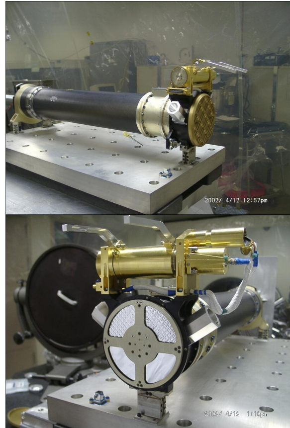
Fig. 49: Inspection of the optical filters of the EUVI Engineering Test Unit (ETU) after vibration testing. Top: EUVI ETU with SESAME in closed position, protecting the filters. Bottom: Opened SESAME, showing that the thin aluminium filters were successfully protected by SESAME.
