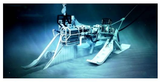
Figure 3-4. Example of a marine plough (Primo Marine, 2022).
