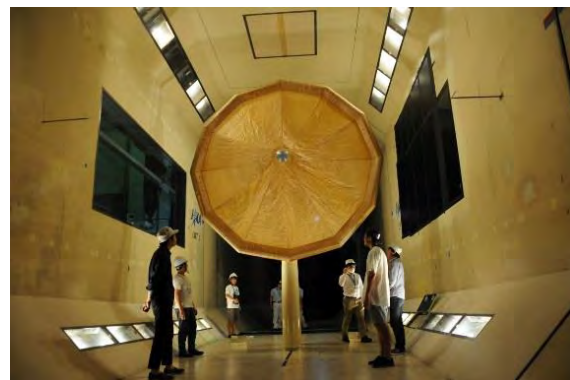
Fig. 2: The mock-up of inflatable aeroshell sustained by single inflatable ring with a diameter of 3.5m.
