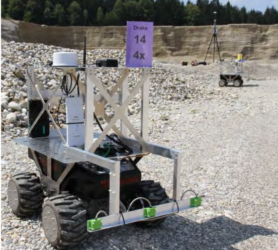
Fig. 1: One of six rovers equipped with DLR's swarm navigation system. The rover is located in a large gravel pit as analog experimentation site.
