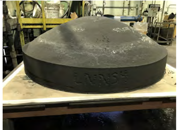
Figure 1. Near net shape cast 1.4m diameter FiberForm Preform.
