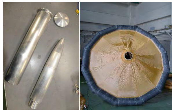
Fig. 1. Half model of Martian penetrator and strage case of this probe (left side) 2.5 m deployable inflatable aeroshell (right side)
