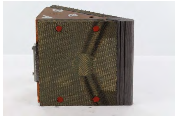
Figure 2. Pre-test image of a seamed HEEET test article.
