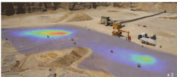
Fig. 2: Start of the gas exploration: two gas sources were simulated together with wind coming from the right. The gas concentration field is shown as overlay.
