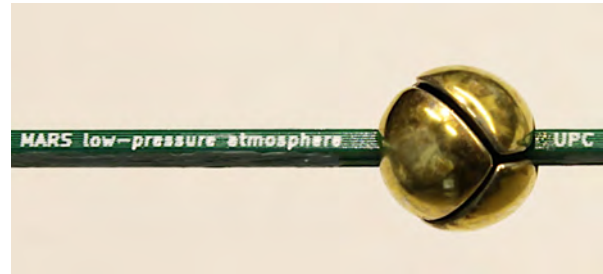
Fig. 1: Photograph of the 4-sector spherical sensor (10mm diameter).
