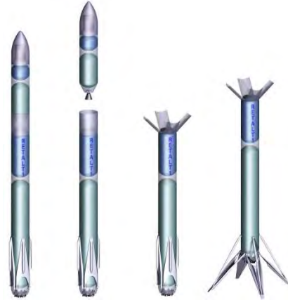
Figure 1: Conceptual sketch of the RETALT1 spacecraft. Configurations from left to right: launch, stage separation, first stage descent, first stage landing.
