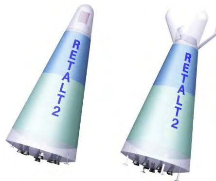
Figure 2: Conceptual sketch of the RETALT2 spacecraft. Configurations from left to right: launch, descent and landing.
